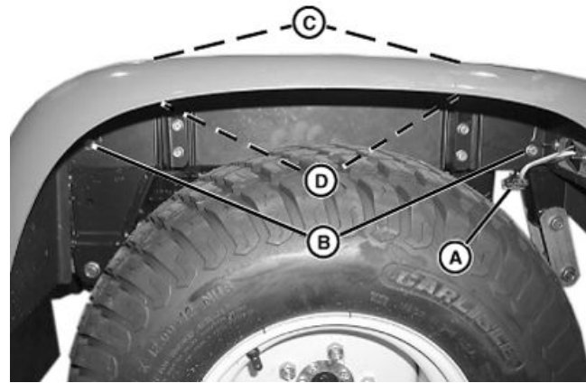
A—Taillights B—Cap Screws
