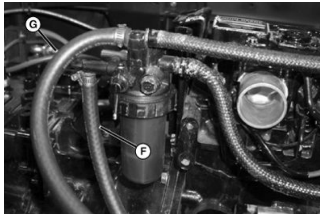
Fuel filter/water separator shown in the open position.
